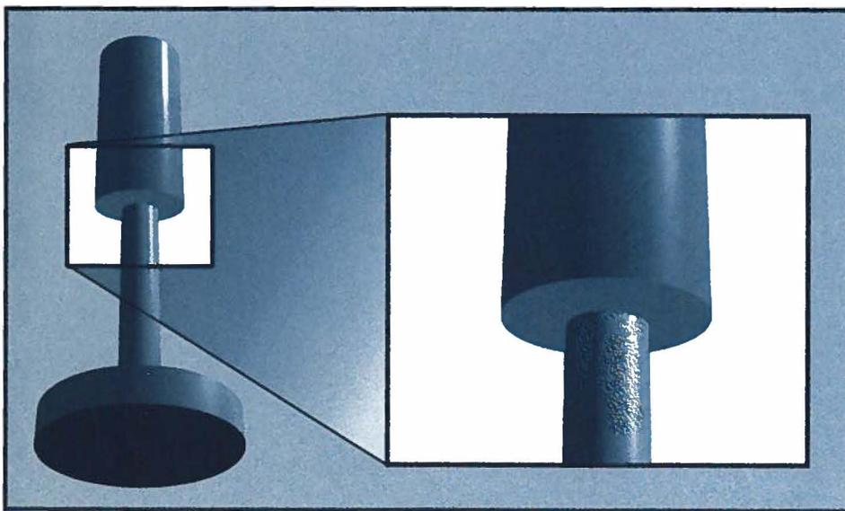
*Under certain water conditions mineral deposits may form on the sliding surfaces of the relief valve. This may cause the relief valve reading to vary, depending upon the amount of deposits*
